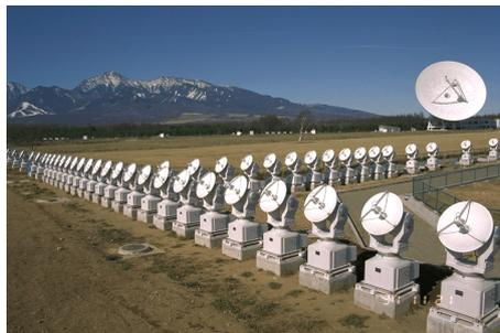
Figure 4.6: The Nobeyama radioheliograph is a traditional T-shape array of telescopes, in the future Frequency Agile Solar Radiotelescope (FASR) will consist of telescopes in no particular array form.
