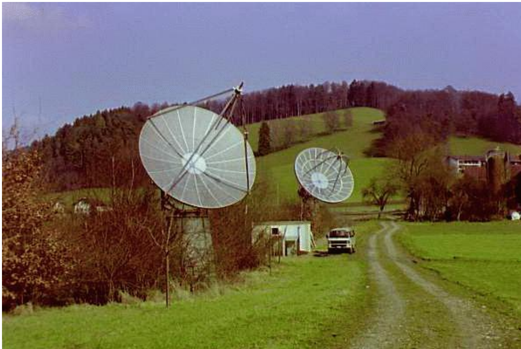
Kuva 4.24: ETH Zürich antennae (Switzerland), operating the Frequency-agile radio spectrometer Phoenix-2
